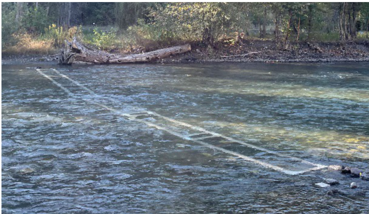
Image above: PIT antenna installed along the bottom of Portage Creek
